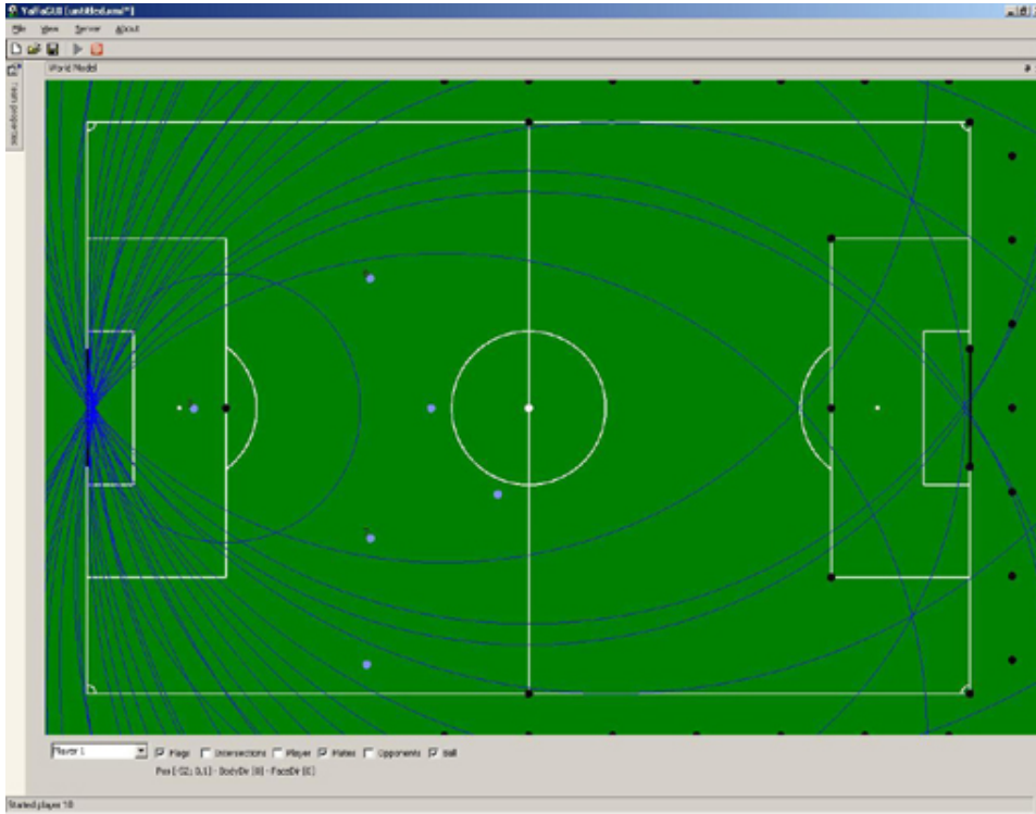
Figure 4.2: Visualization of the world model where the position of the selected player, the distance to the seen flags, the team mates and the ball is displayed.
